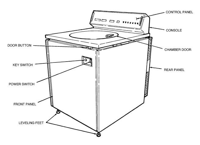
Figure 1-1 Centrifuge Parts Location and Identification
