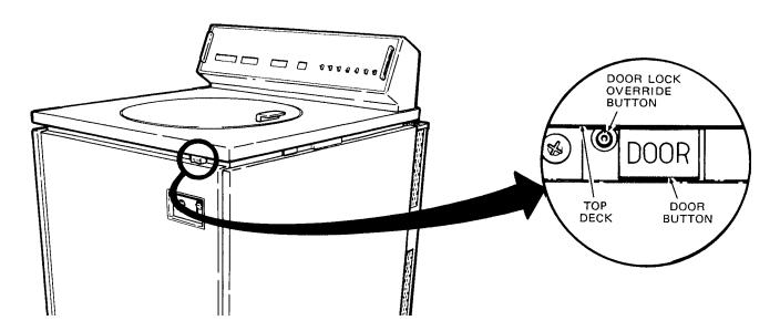
Figure 4-1. Door Latch Override Button Location
