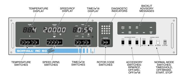
Figure 3-1. RC-5C PLUS Control Panel
